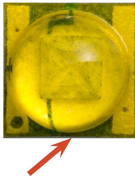
It is not required to use a solder footprint for the thermal pad that is larger than the XLamp XT Family LED itself. In testing, Cree LED has found such a solder pad to have insignificant impact on the resulting  $T_c$  measurement.
